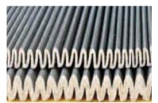
Photo above shows 'dry' Par-Gel filter media and the same media swollen with absorbed water
