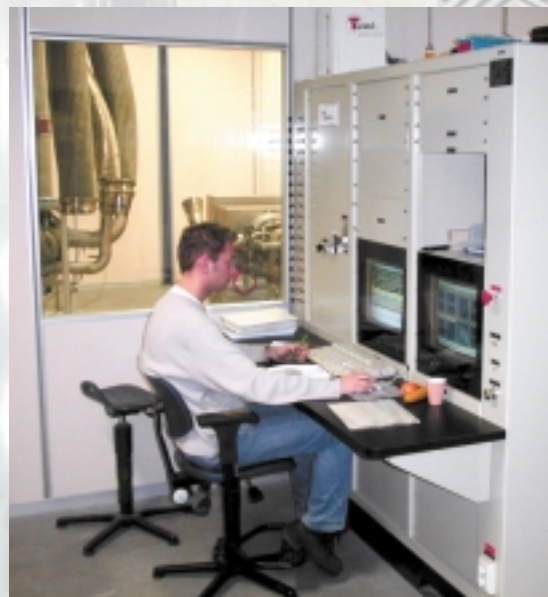
Typical computer-aided pneumatic test cell console, showing test unit behind the window. Twin color display screens allow the operator to see the test program and real-time data on one screen, test report generation and setup graphics on the second screen. User-friendly TestEx software constantly monitors operation of the test part and test cell for out of range or unsafe conditions.
