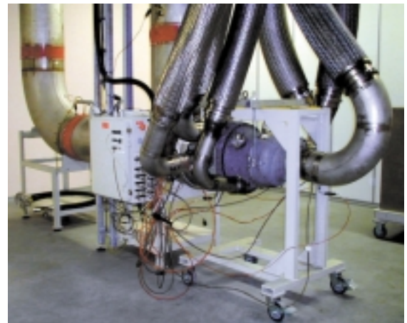
Interior view of air cycle machine test cell adapted to test Boeing 777 ACMs. Note use of cart for safe test part handling; this also increases test efficiency by allowing technicians to set up one cart/test unit while another is being run in the test cell.
